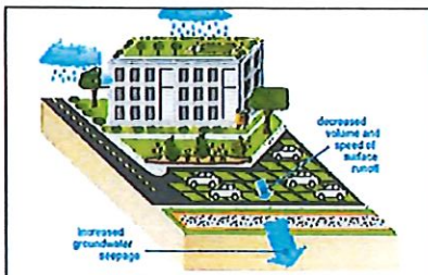
Green areas incorporated into impervious areas reducing runoff
